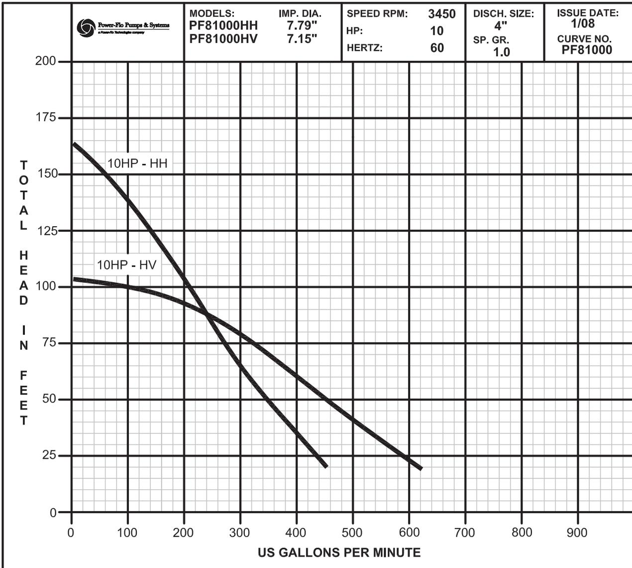
Dewatering Pumps - 10HP - 3450RPM - 60Hz
