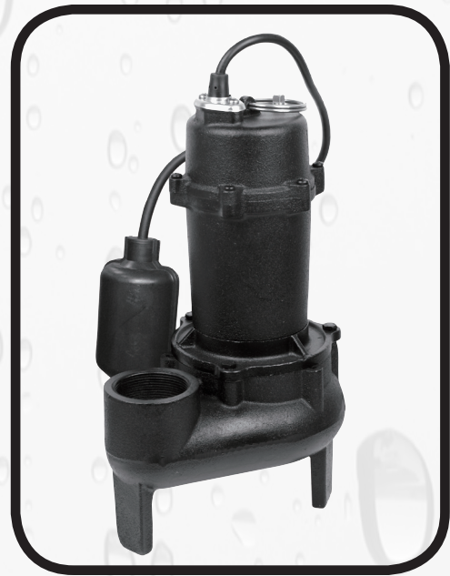
Submersible Sewage Pump 1/2HP, 115V 2" Discharge, 2" Spherical Solids Cast Iron Wide Angle Tethered Float
