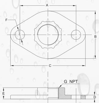
Circulator Flange 3/4", 1", 1-1/4", Threaded, IPS Connection Ductile Iron
