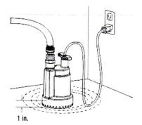
Place the pump on a solid base in flooded area or any place that you would like to remove water. Plug the pump into a 115 volt GFCI power outlet.
