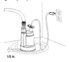
Allow the pump to run and monitor its progress. Unplug the pump when it has removed water down to approximately 1/8 in. Remove the pump and hose from the location when finished pumping. The hose still has water that can drain back through the pump. Remove remaining water with a squeegee, mop, sponge, towel, wet/dry vac, etc.
